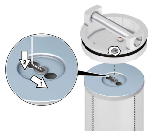
Fig. 5: Removing the filter element from the cover
